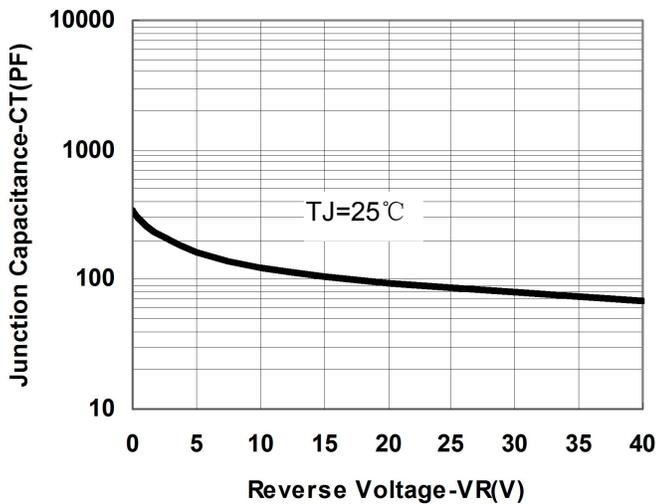
Fig.1-Typical Junction Capacitance
